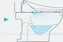
The sterilizing water comes out from the nozzles and is sprayed into the bowl.
